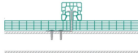
Section panels joining with aluminum snap-on profile.
